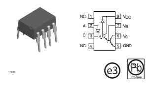
Photo darlington operation is achieved by tying the  $V_{CC}$  and  $V_O$  terminals together. Access to the base terminal allows adjustment to the gain bandwidth.
