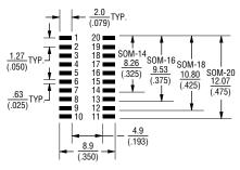
NOTE: Land pattern dimensions are based on design rules established by the Institute for Inter-D connecting and Packaging Electronic Circuits in [] IPC-SM-782
