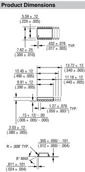
Lead coplanarity .102mm (.004 inch) max. at mounting surface.
