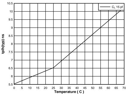
Figure 1. Propagation Delay vs Temperature
