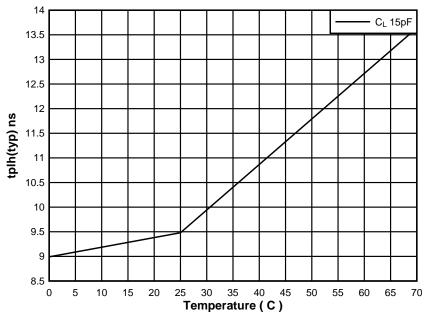
Figure 4. Propagation Delay vs Temperature
