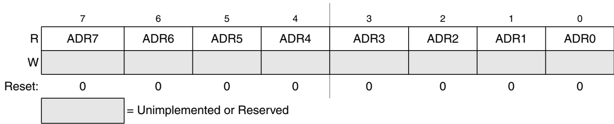
Figure 14-7. Data Result Low Register (ADC1RL)
