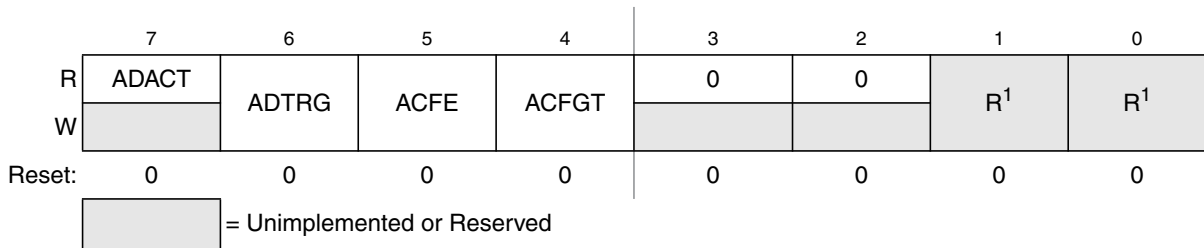
Figure 14-5. Status and Control Register 2 (ADC1SC2)
